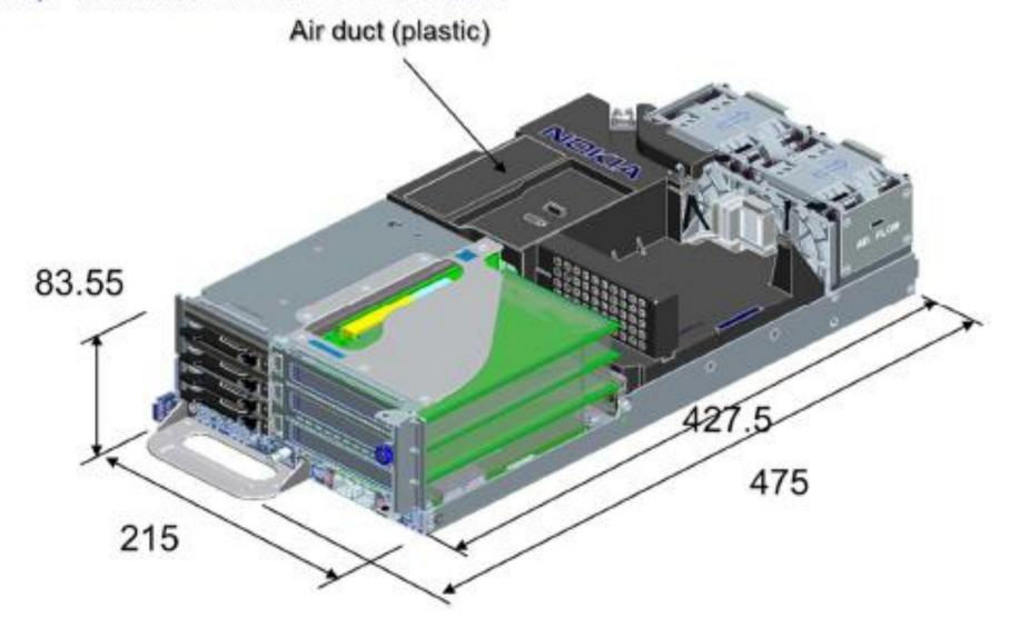
Dimension 475 mm x 215 mm x 41 mm (DxWxH). It can support below configurations:
